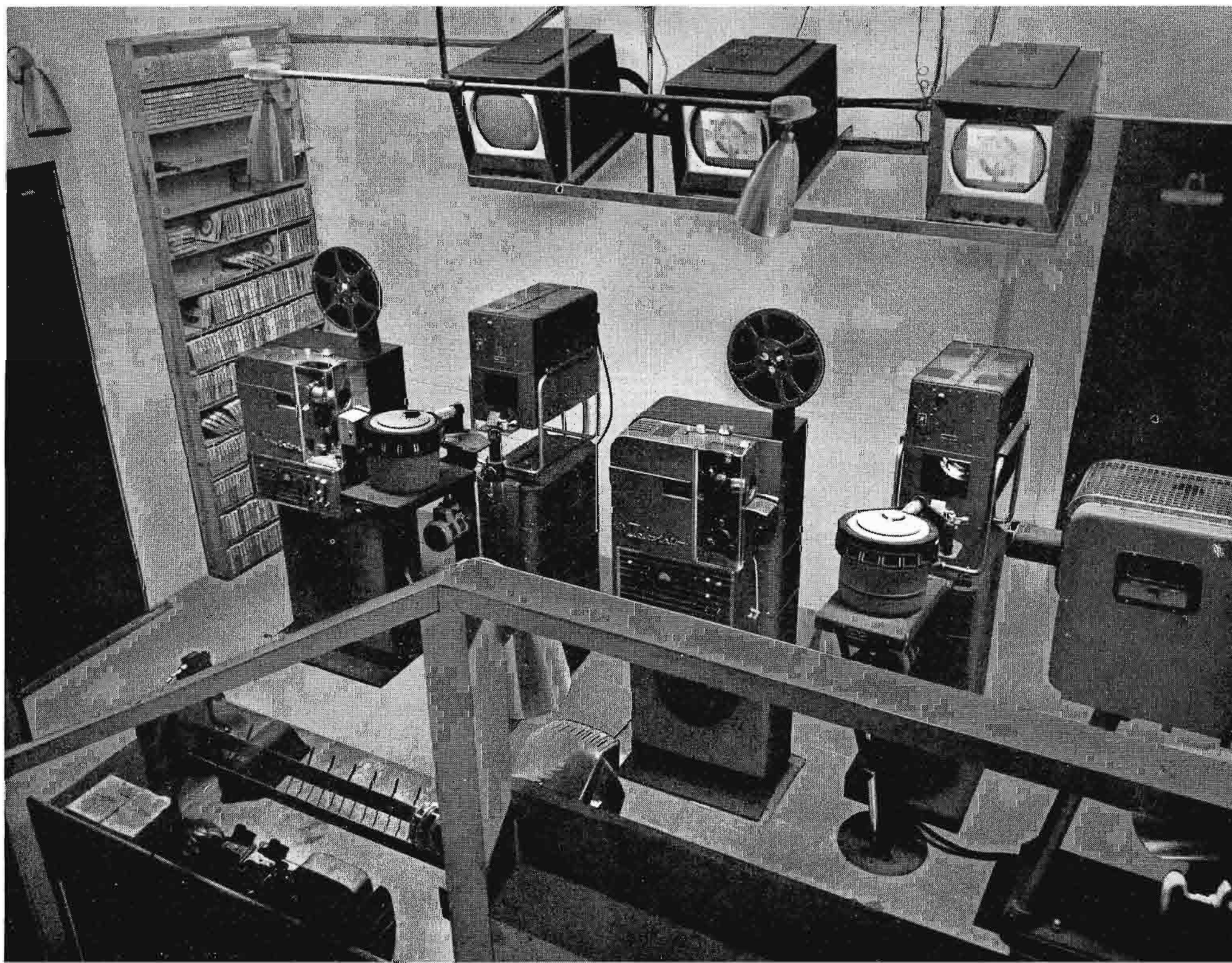
FIG. 17. View of WSUN-TV film room. Two RCA TP-6A Professional Film Projectors are shown, each with an individual TK-20D Film Camera. Multiplexed with the film projectors are two automatic slide projectors, and to the right, a Gray Tel-Op. Above are three RCA Utility Monitors.
