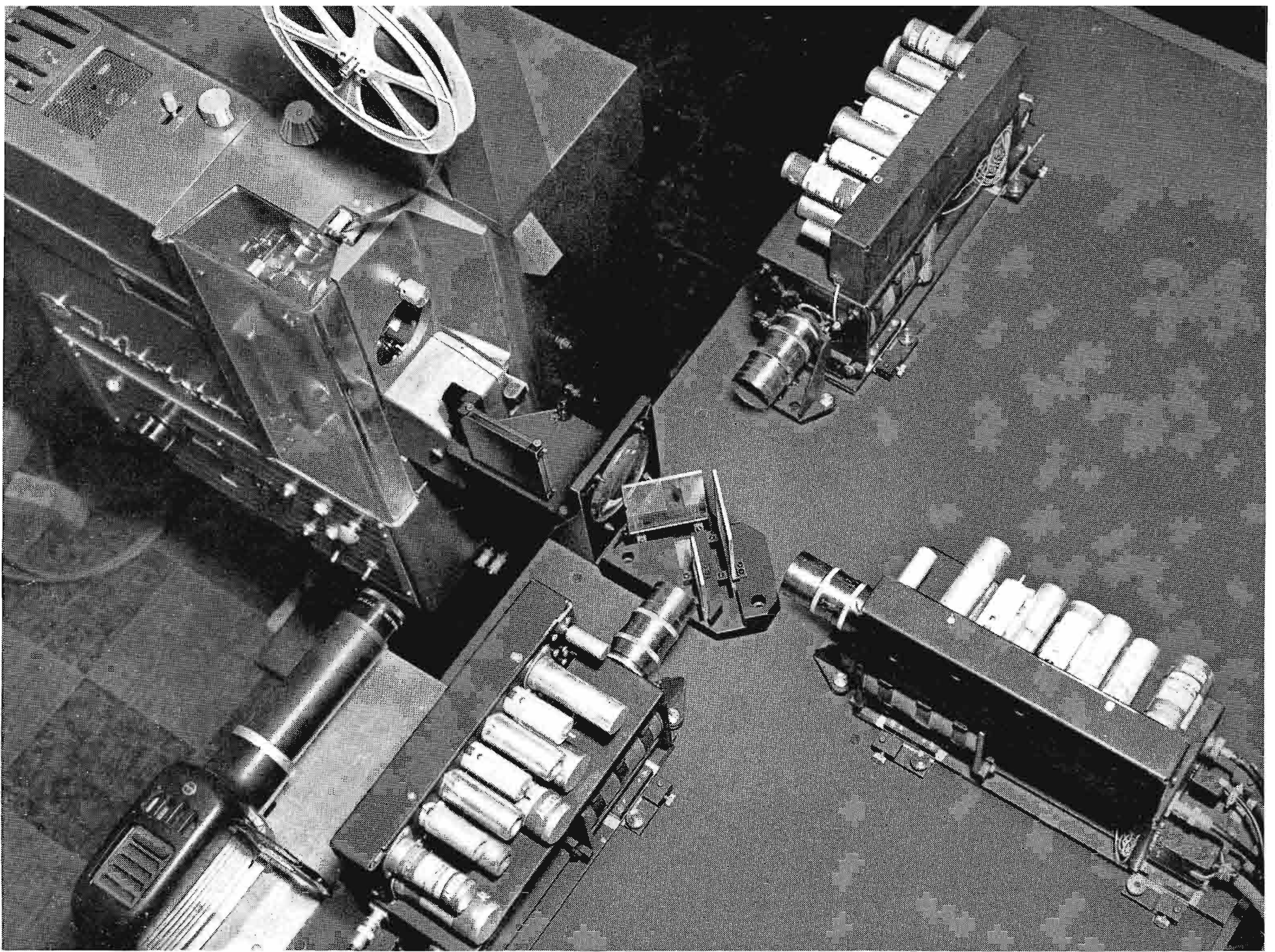
FIG. 3. Close-up view showing blue, green and red vidicon chassis and dichroic mirror system.
